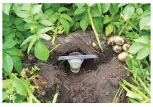
Figure 28 Measuring flow rate from emitters along a drip line a) surface line on grape vines b) buried line on potatoes
