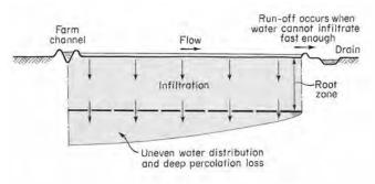
Figure 21 The surface irrigation problem
