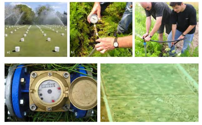
Figure 26 Sprinkler evaluation a) measuring uniformity b) pressure c) discharge from a sprinkler d) flow meter on mainline e) doughnut ring effect in crop when pressure is too low
