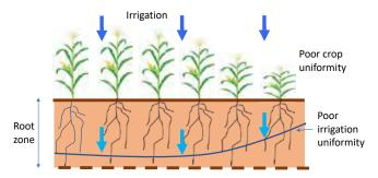
**Figure 6** Three different ways of measuring efficiency: Water application efficiency = 100%; Water distribution efficiency = 80% Water storage efficiency = 75%
