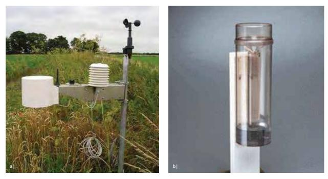
Figure 30 Tools for irrigation scheduling a) automatic weather station b) rain guage
