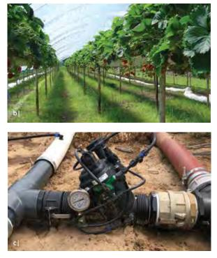
Figure 27 Drip irrigation a) on field scale crops b) drip on protected fruit crop c) pressure control equipment
