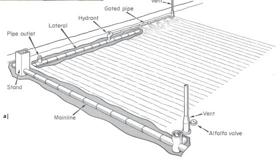
Figure 14 a) Low-pressure pipe system for surface irrigation b) gated pipe used to irrigate furrows.
