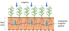
Figure 4 Inadequate irrigation, but the efficiency approaches 100%
