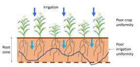
Figure 5 Impact of poor irrigation uniformity on efficiency and crop growth
